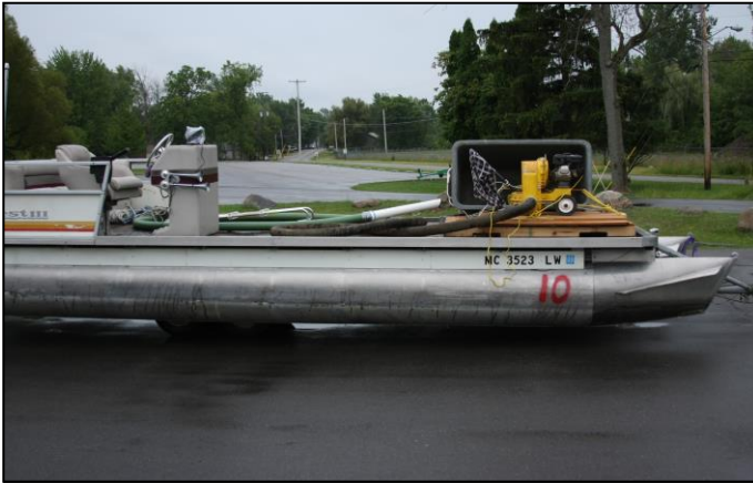
Figure 67. A DASH boat for hand-removal of milfoil or other nuisance vegetation. ©Restorative Lake Sciences
